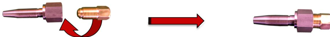
3. Put a little grease on the tip of the stainless steel cone and screw it by placing it straight in the brass fitting. Stop as soon as the stainless steel thread has disappeared in the brass nozzle, i.e. about 7 mm of space between the nut and the brass fitting.
